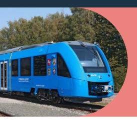
Coradia iLint is a full emission-free train solution based on Alstom's successful Coradia Lint platform. The traction system is using fuel cells which produce electricity by combining hydrogen and oxygen to water.
