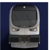
The loco structure is made of high-strength steel. Side covers and removable roofs are made of light alloys.
